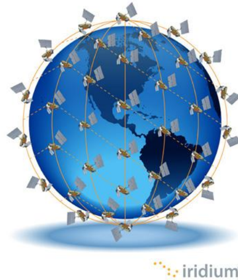
Image illustrates how a constellation of communications satellites provides global coverage. Image c/o Iridium.
