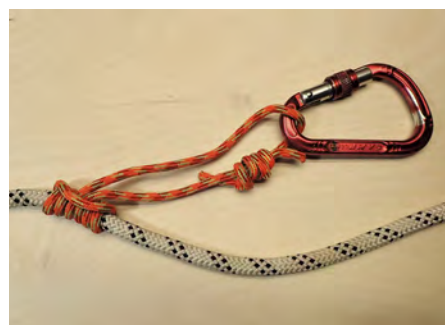
Figure 4. A dressed, three-wrap prusik hitch.
