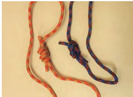
Figure 1. Two prusik loops, one tied with a double fisherman's knot (left), the other tied with a figure-eight bend.
