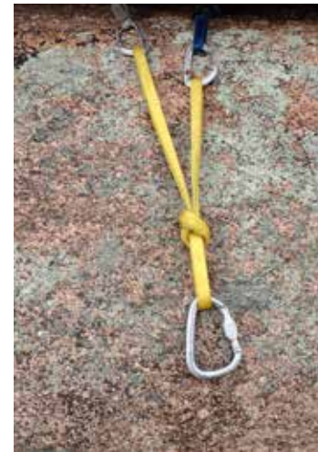
Figure 6. Completed ponytail anchor.
