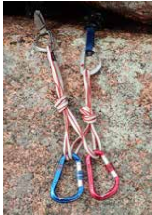
Figure 8. Completed quad anchor with double master point.
