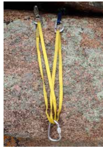
Figure 3. Completed magic X anchor with locking carabiner at the master point.
