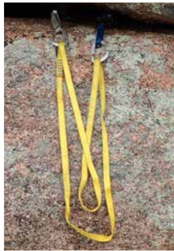
Figure 2. Twisted strand for a magic X anchor.
