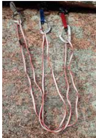
Figure 9. Triple-length sling clipped to three POA to start a three-point ponytail anchor.
