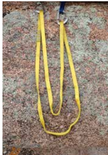
Figure 5. Clipping a sling into each POA to start a ponytail anchor.
