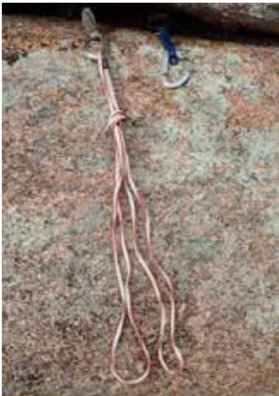
Figure 7. Triple-length sling doubled, knotted, and clipped into one POA to start a quad anchor.
