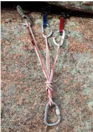
Figure 10. Completed three-point ponytail anchor.
