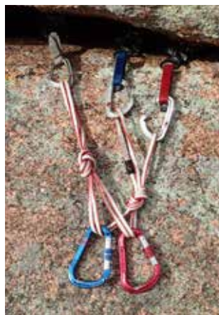
Figure 12. Completed three-point quad anchor.
