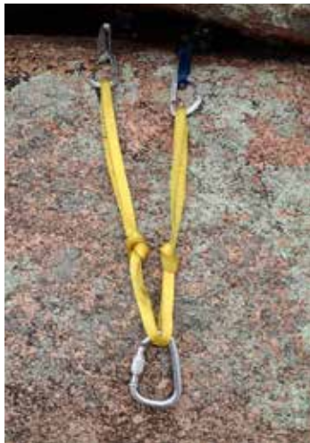
Figure 4. Magic X anchor with extension-limiting knots.
