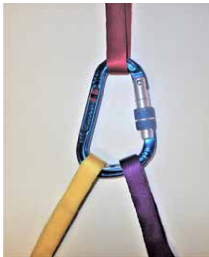
Figure 3. Triaxially loaded carabiner.
