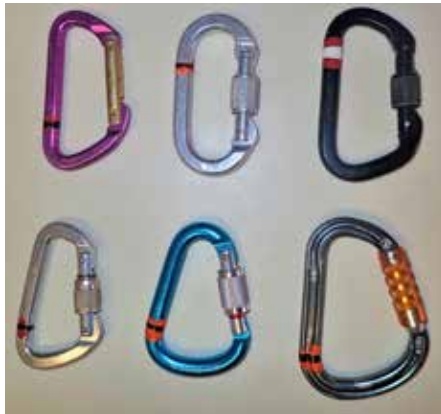
Figure 2. Assortment of carabiner shapes. Clockwise from upper left: nonlocking D-shaped carabiner, locking oval carabiner, locking D-shaped carabiner, triple-action autolocking pear-shaped carabiner, screw-lock pear-shaped carabiner, and asymmetric locking D-shaped carabiner.
